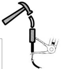
Fig. 4: Remove old cable sheathing.
